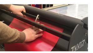
Open the clamp and place your transfer into your TW17. The liner should be facing downwards. Close the clamp so your transfer is hold firmly in place.
