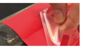
Now the transfer is stuck to the core, you can pull the liner away from the transfer down towards your working table.
