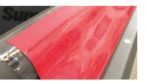
Pull the media to the core of your TW17, and stick the top of the transfer to the tape on the core.
